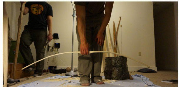
Bow being pulled- notice the lack of bend in outer limbs and overbend just past the right fadeout. This is accentuated by the perspective of the photo, though still needs attention moving forward.
