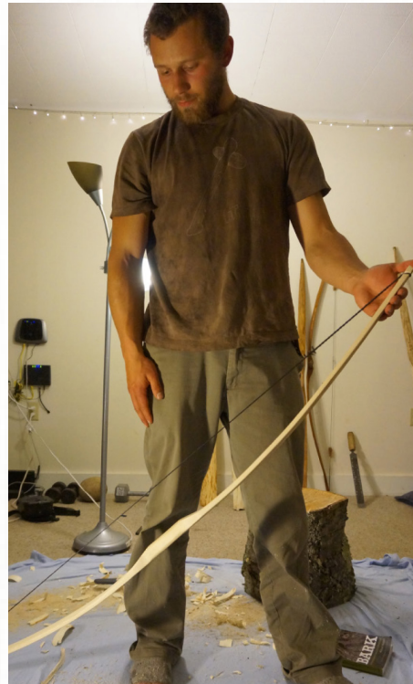
Ease off and let the string settle into the bow. Be sure to check your nocks to make sure the string is securely in.
