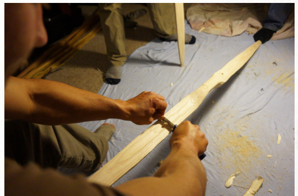
Another view of using a knife as a scraper on the belly of the bow
