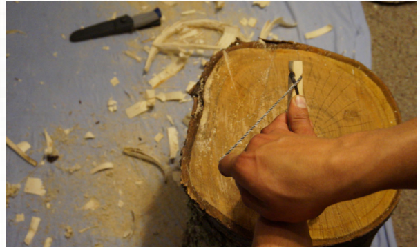
Tying a timber hitch knot
