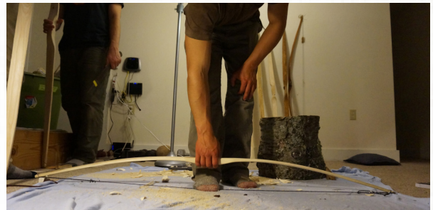
Stepping on the string and pulling up on the handle of the bow allows an observer to get a good view of the bow.
