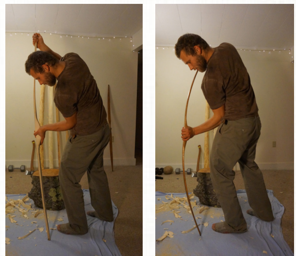
Floor tillering: (left) showing a stiff bow blank, (right) showing deeper bend from a finished bow
