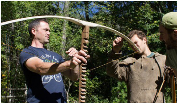
Observing the tiller on a tillering stick
