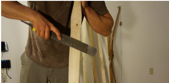
Using a rasp on the belly of the bow
