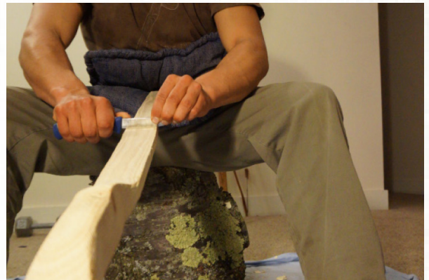
Using a knife as a scraper on the belly of the bow. A pillow is in between my stomach and the bow, allowing me to work towards myself
