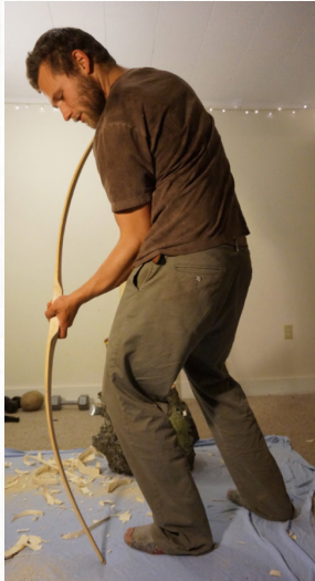
Another look at the floor tiller. These pictures are showing both limbs of a finished bow. Notice the smooth, even curve throughout the limb.
