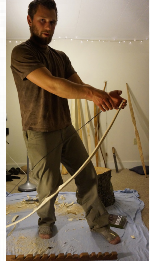
Lean your knee onto the handle of the bow while pulling up on the tip, this ensures bending the bow evenly as we string it.
