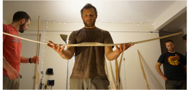
Bow at a brace height. Observing the negative space between the bow and the string is a great tool for observing tiller.
