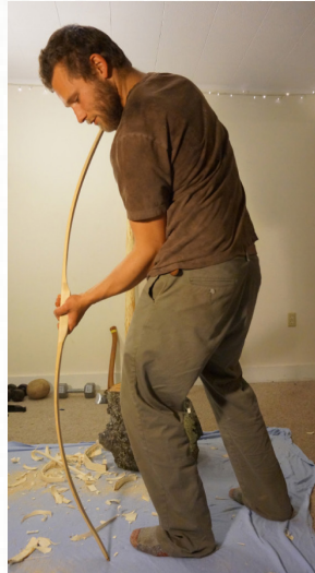
Another look at the floor tiller. These pictures are showing both limbs of a finished bow. Notice the smooth, even curve throughout the limb.
