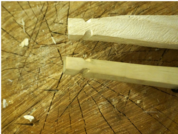
Picture of nocks on a bow blank (top) and finished bow (bottom)
