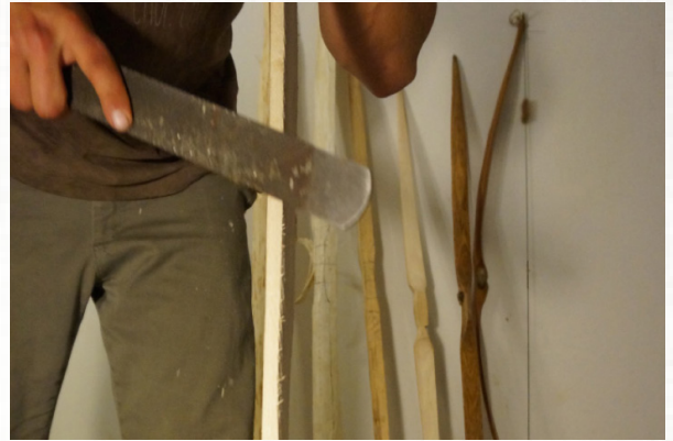
Using a rasp on the side of the bow, being sure to keep the sides perpendicular to the belly
